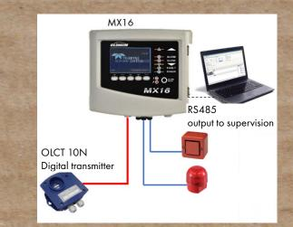
With its 3 relays available (AL1, AL2 and fault), a graphic screen that allows you to read values such as:
