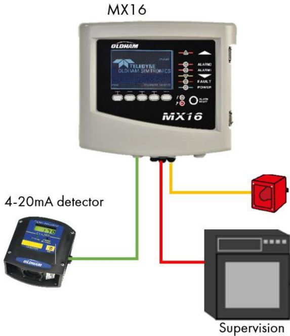
Figure 2: Example of an MX 16 configuration using one analog detector
