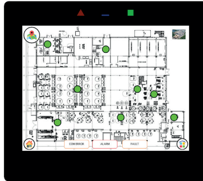
Gas detection layout on-site
