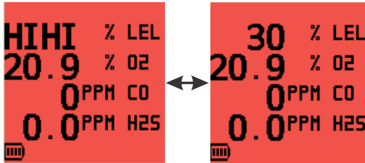
Figure 4-2: LEL HIHI Alarm
