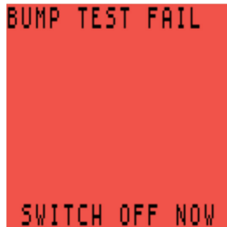
Figure 6-8: Bump Test Fail - Switch Monitor OFF
