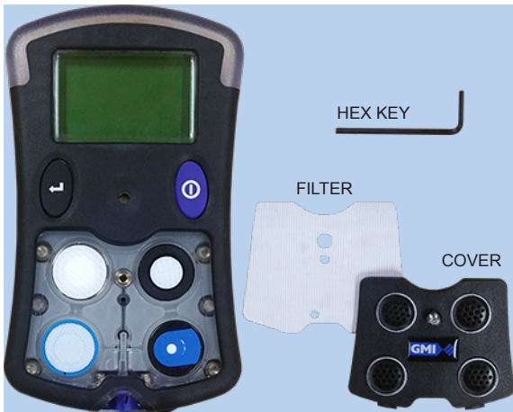
Fig. 4.2 Filter and Cover Removed
