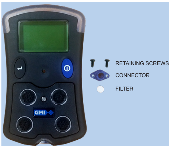
Fig. 4.4 Filter and Connector Removed
