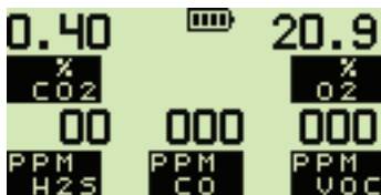
Abb. 3.7 CO 2 -Sensor - Zero Fault
