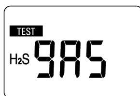
Figure 4-2: Manual Bump Test - Apply Gas
